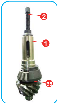
Remove the big bearing of mainshaft: 拆除主軸大培林:
