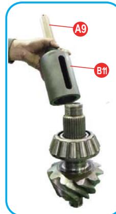
Install the big bearing of mainshaft: 安裝主軸大培林:
