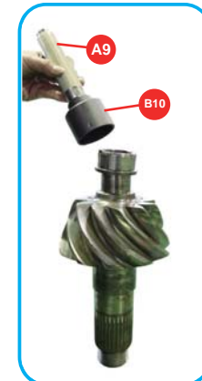
Install the inner sleeve of mainshaft: 安裝主軸培林內套管:
