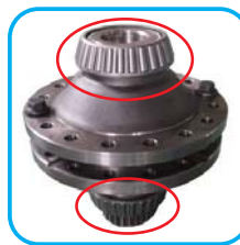
Install the differential front bearing: 安裝差速器前培林
