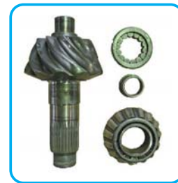
Install the differential rear bearing: 安裝差速器後培林
