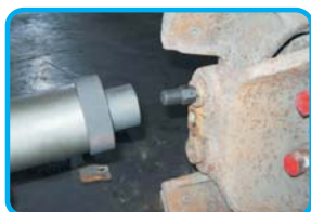
1. Connect anchor pin extractor with anchor pin and cylinder fixation. 把來令片插銷、油壓缸固定座和來令片插銷拔卸器連結。
