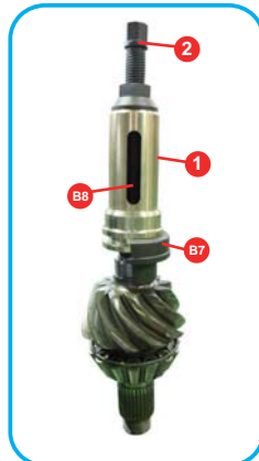
Remove the inner sleeve of mainshaft: 拆除主軸培林內套管:
