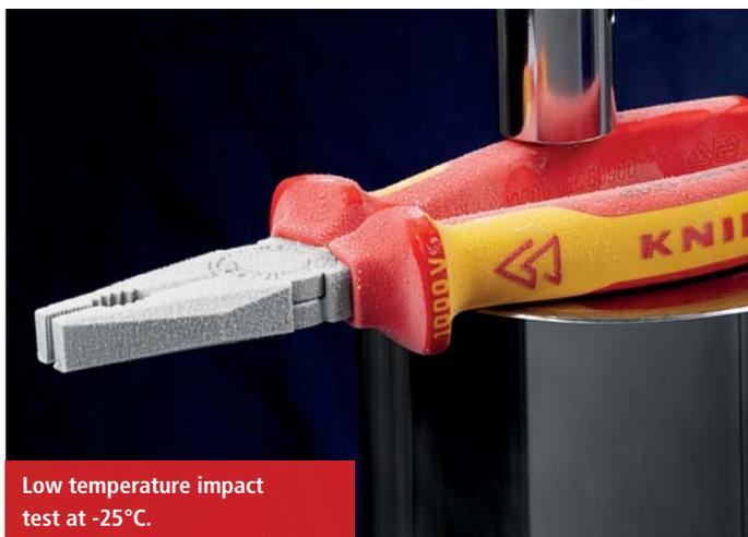
Low temperature impact test at -25°C.
