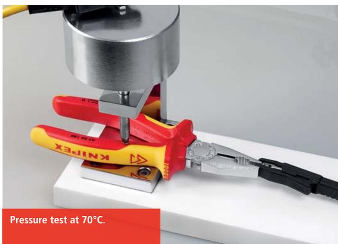
Pressure test at 70°C.
