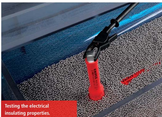
Testing the electrical insulating properties.
