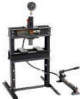
Манометр и выносной насос/Pressure gauge and remote-mount pump
